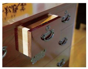
Precise workmanship creates the unique air-tight construction of traditional Japanese bureaus, or *tansu*. The fit is so tight that when a drawer is pushed in, air pressure will push it back out. This incredible precision is the result of a production process in which a single traditionally trained cabinetmaker performs every task, from cutting logs into boards to assembling the furniture.
