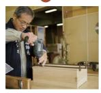
Use a drill to make a hole for the wooden nail in the bottom of the drawer.
