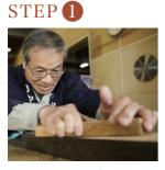
Hold the plane firmly and press it down hard on the wood surface.
