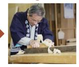
Keep pressing down and pulling to the very end. Feel the surface of the wood — it's changed from rough to silky smooth.
