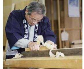
Keep pressing down and pulling to the very end. Feel the surface of the wood — it's changed from rough to silky smooth.
