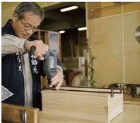
Use a drill to make a hole for the wooden nail in the bottom of the drawer.
