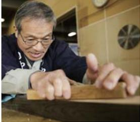
Hold the plane firmly and press it down hard on the wood surface.
